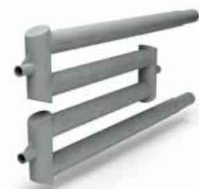
U- and W-shaped radiant tubes for tube temperatures up to 1250°C (2280°F). The Kanthal program of U- and W-shaped radiant tubes includes nickel-chromium (NiCr) alloys or Kanthal APM™ and Kanthal APMT™ iron-chromium-aluminium (FeCrAl) alloys for extremely demanding environments, or as hybrid solutions with combinations of the different material types for maximized performance.
