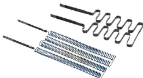
Ready-made metallic heating elements made from wire or strip in Kanthal® iron-chromium-aluminium alloys or Nikrothal® nickel-chromium alloys.
