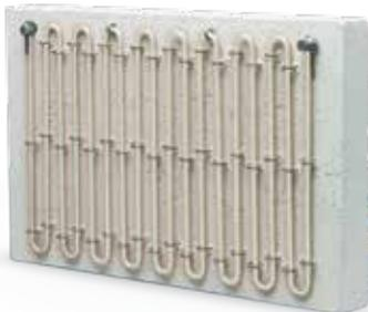
Prefabricated heating modules with metallic heating elements and non-electrically conductive, dense ceramic insulation for use at element temperatures up to 1350°C (2460°F). The construction method of Moduthal™ heating modules ensures accurate positioning of the elements and eliminates the distortion or other problems connected to the conventional open coil elements in grooves or on tubes.
