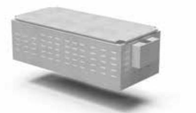
The Kanthal highly focused reflector-based electric heating solution ensures more thorough drying. Kanthal reflector technology is uniquely designed to provide focused radiation into the stub holes only, and not on the anode block itself. This means that significant energy savings can be achieved.
