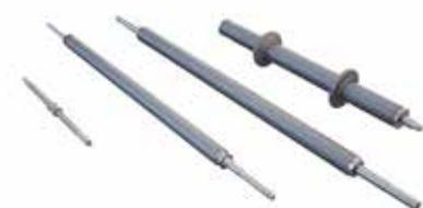
Our sophisticated Kanthal APMT™ rollers ensure the best performance in critical 'hot zones', with operating temperatures up to 1250°C (2250°F). Kanthal APMT™ furnace rollers provide longer service life compared to conventional materials, for high temperature and demanding applications. Kanthal furnace rollers are available in outside diameters from 26 to 260 mm (1 to 10 in.), according to customer design.
