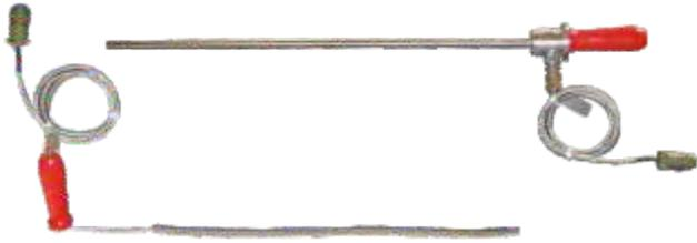
Hot Bolt Heaters are used to preheat large, hollow holding bolts or studs where a high concentration of heat is critical for bolt expansion in a short period of time.
