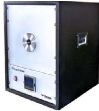
Black bodies are reference sources used for testing infrared systems. They are required in industry for calibration of pyrometers, infrared line scanners or cameras.
