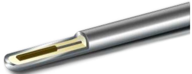
Self-Powered Neutron Detectors are in-core flux monitors in nuclear power reactors. The typical SPND is a coaxial cable consisting of an inner electrode (the emitter), surrounded by insulation and an outer electrode (the collector).
