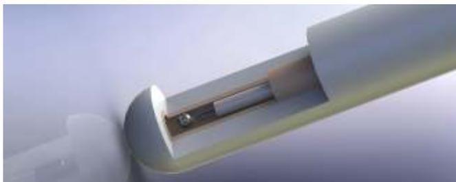
Thermocouple Insert Construction
