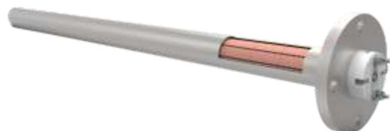
Marathon Tempwatt make Ceramic Bobbin Heaters are fabricated from high temperature refractory insulators in various diameters and lengths for any voltage or wattage within manufacturing limits. These Bobbin Heaters consist of elements, which are exposed partially in air for better transmission of heat. Also, when it is inserted into a thermowell, it offers a large heated area to the liquid or semi-solid to be heated.
