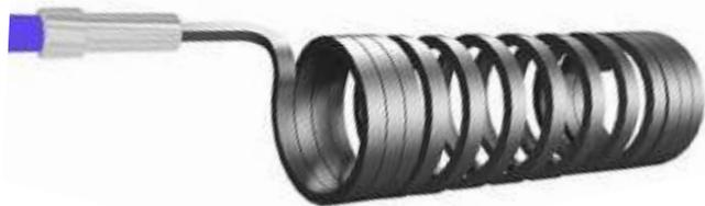
The basic construction of these heaters consist of compacted MgO, high temperature resistance wire and Chrome Nickel Steel tube. These heaters can be constructed with or without built in thermocouples.
