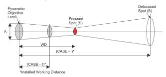
Case-I: If installed working distance is greater than manufactured working distance
