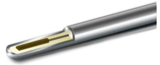
Self-Powered Neutron Detectors are in-core flux monitors in nuclear power reactors. The typical SPND is a coaxial cable consisting of an inner electrode (the emitter), surrounded by insulation and an outer electrode (the collector).
