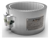
• Ceramic band heaters are medium-to-high temperature heaters that have 550°C as the maximum working temperature. These durable heaters can have optional in-built ceramic fiber jackets that make them energy efficient. Ceramic band heaters are available with different terminal styles, are fully flexible, and can accommodate holes and cut-outs.
