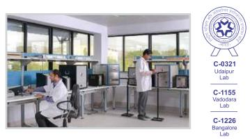
The calibration center functions as per ISO 17025 / NABL standards. Calibration of contact type sensors can be made in temperature range of -196°C to 1600°C.and Calibration of non contact type sensors can be made in temperature range 0°C to 2700°C. Further the laboratory is accredited for onsite temperature calibration.
